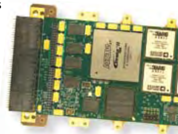
Based on the Altera Stratix family of FPGAs for signal processing
